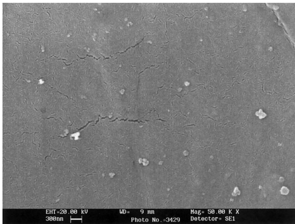
Figure 15 SEM micrograph of the 2 wt % organo-MMT nanocomposite (original magnification, 50,000 \times ).
